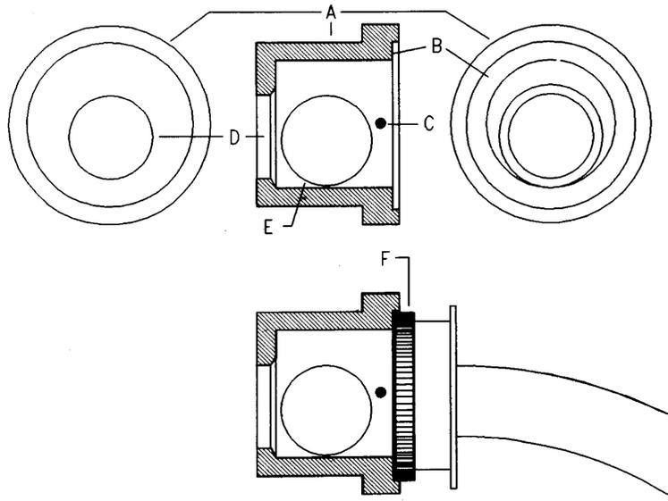
Fig 1. Cross section of ball valve connected to a No. 6 Jackson metal inner cannula. A, Valve body; B, recess into which the cannula flange fits; C, ball stop, which prevents the ball from entering the cannula; D, combination input port and valve seat (note that this is not concentric with the axis of the valve body); E, ball; F, flange on a Jackson low-profile metal inner cannula.
