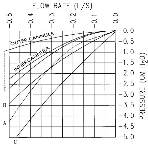
Fig 6. Airflow characteristics of the Shiley (B), Passy-Muir (C), and ball valves (A) as they are attached to the inner cannula of a No. 6 Shiley tracheotomy tube, and of the ball valve (D) as it is attached directly to the outer cannula of a No. 6 Shiley tracheotomy tube. These are compared with the airflow characteristics of the outer cannula and the inner cannula alone.
