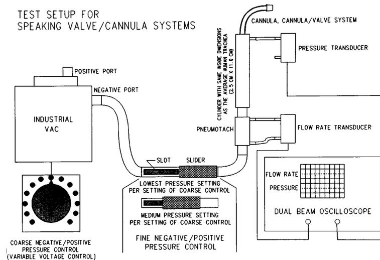
Fig 5. Diagram of pneumotachometer used to measure the inspiratory and expiratory flow characteristics of the speaking valves.
